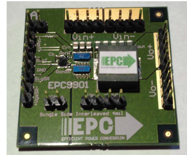
Prototype L_{LOOP} \approx 0.4 \text{ nH}
